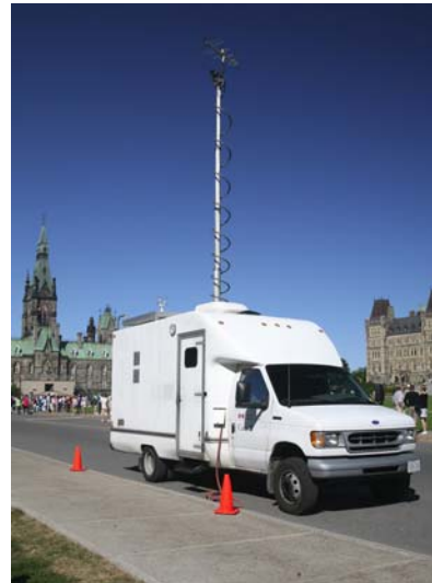
Fig 5. Mobile Transmission Laboratory for television transmission and coverage tests (Picture shows tests being carried out at Parliament Hill in Ottawa)
