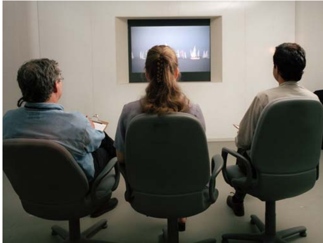
Fig 2. Viewing Room of ATEL. The lighting level and colour of the back-lit viewing wall meets the requirements of ITU-R Recommendation 500. Viewers are seated at a distance as is appropriate for HDTV or Standard TV.
