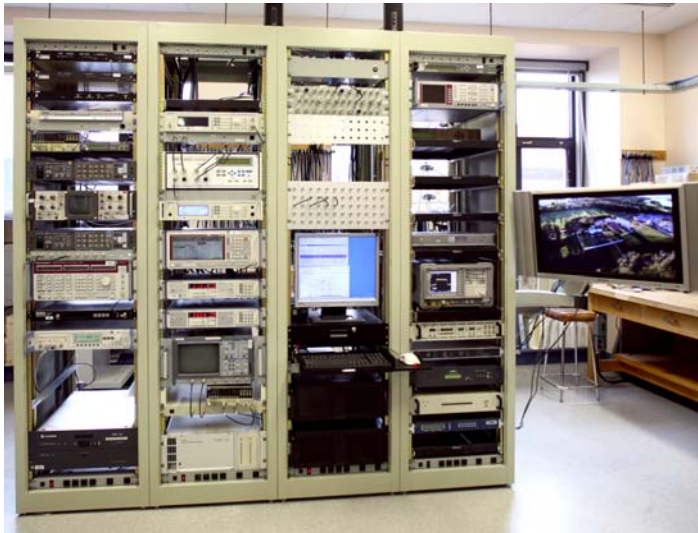
Fig 4. Equipment at the Transmission Laboratory to simulate transmission environments for testing and comparing robustness to transmission impairments of different transmission and modulation technologies
